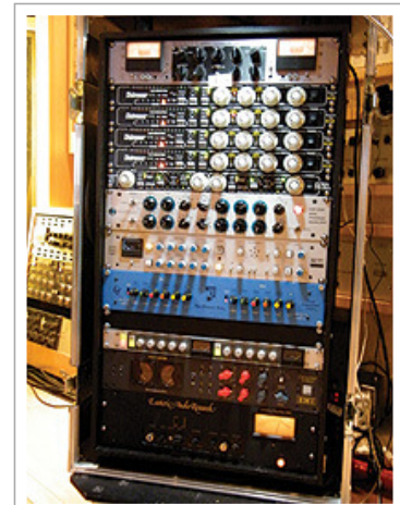
A small selection of Cenzo Townshend's vast array of outboard, including several items used on his mix of 'You've Got The Love'. From top: Manley Vari-mu compressor, Empirical Labs Distressor compressors (x4) and Fatso tape emulator, Summit EQP 200B equaliser, SSL XLogic compressor, NTI EQ, Smart C2 compressor, Chandler/EMI TG1 limiter and EAR 660 compressor.
